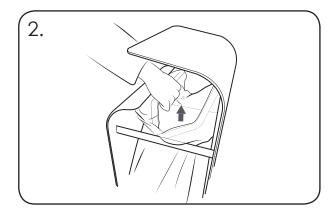
Feed the sack up through the sack bands from beneath. Wrap the top of the sack over both bands.
